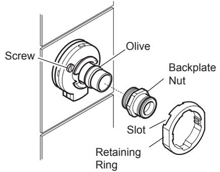
11. To prevent the backplate from turning while tightening the nut, fit the retaining ring over the backplate nut making sure the slots engage with the screws on the backplate, hold the retaining ring with a wrench while tightening the backplate nut. Remove the retaining ring after use.
