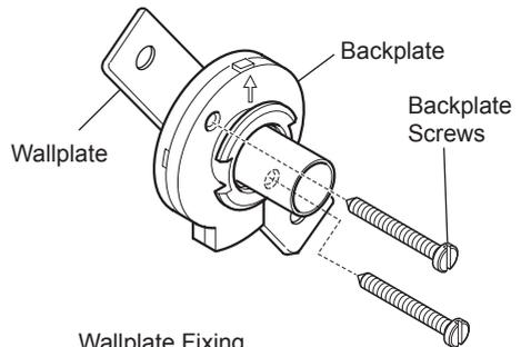
4. Place the backplate/wallplate assembly over the copper pipe with the arrow pointing up. The screw holes should be at 40° to the horizontal.
