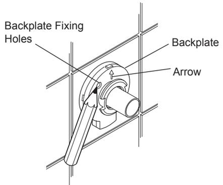
8. Place the backplate over the copper pipe with the arrow facing up.
