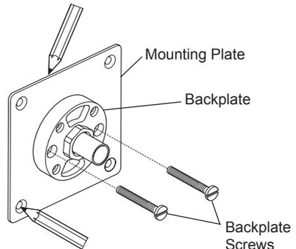
6. Remove the mounting plate/backplate assembly from the wall.
