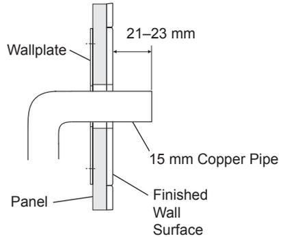
4. Place the backplate over the copper pipe with the arrow pointing up. The screw holes should be at 40° to the horizontal.
