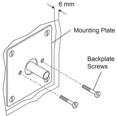
11. Temporarily fit the two backplate screws into the mounting plate. This will prevent the fixing holes from becoming blocked with plaster or grout.
