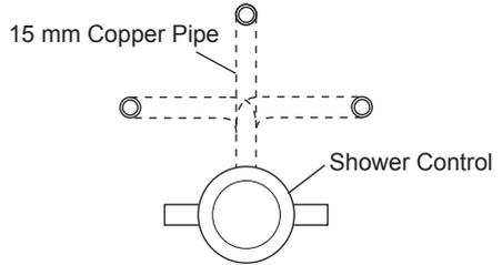
2. Drill a 25 mm hole in the wall for the copper pipework.
