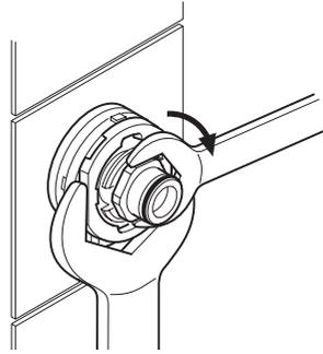
18. Check that the second 'O' seal (black) is fitted to the outside of the backplate nut. Press the elbow onto the backplate, make sure that the clips on the elbow engage with the backplate.
