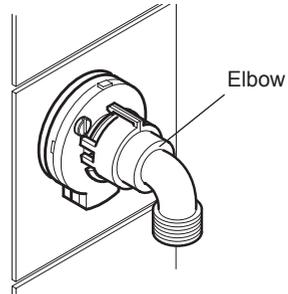
14. Press the shroud over the elbow, make sure that it engages with the lugs on the backplate.
