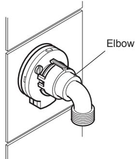
19. Slide the retaining ring over the elbow and engage with the elbow clips. **Note!** The retaining ring must be engaged correctly to lock the elbow to the backplate, rotate the retaining ring to the position illustrated.
