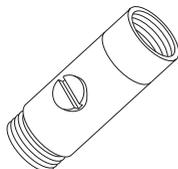
**Outlet Double Check Valve (DCV-H)**
