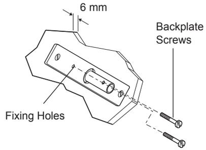
12. Temporarily fit the two backplate screws into the wallplate. This will prevent the fixing holes from becoming blocked with plaster or grout.
