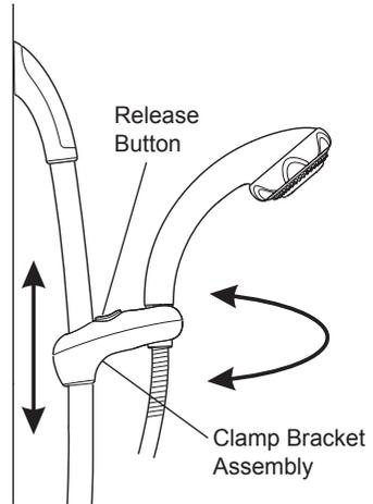
2. Move the handset to the required angle. A friction mechanism within the clamp bracket assembly will hold the handset at the desired angle.
