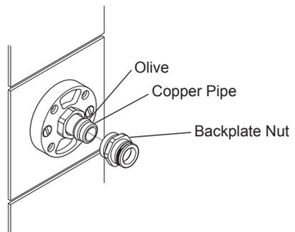
16. Ensure that the 'O' seal is fitted on the backplate nut. Push the BIR assembly over the backplate nut onto the backplate.
