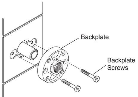
15. Fit the olive over the copper pipe and tighten the backplate nut into position.
