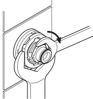
13. Slide the retaining ring over the elbow and engage with the elbow clips. **Note!** The retaining ring must be engaged correctly to lock the elbow to the backplate, rotate the retaining ring to the position illustrated.
