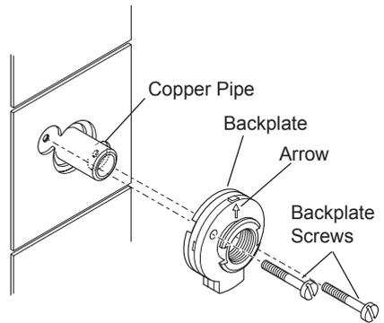
15. Place the backplate over the copper pipe with the arrow facing up and tighten the two backplate screws. Make sure that the foam seal abuts the finished wall surface.
