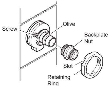
17. To prevent the backplate from turning while tightening the nut, fit the retaining ring over the backplate nut making sure the slots engage with the screws on the backplate, hold the retaining ring with a wrench while tightening the backplate nut. Remove the retaining ring after use.
