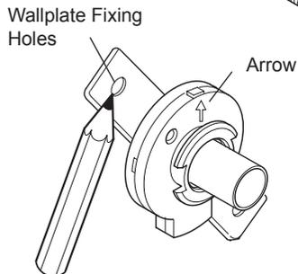
5. Mark the positions of the two wallplate fixing holes.
