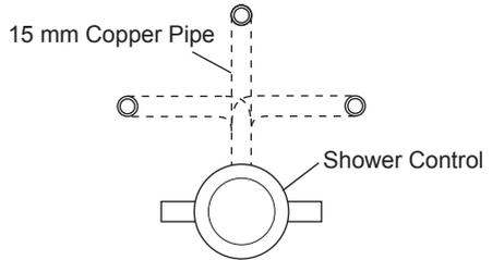
2. The 15 mm copper pipework must protrude through the finished wall surface by **21–23 mm**.
